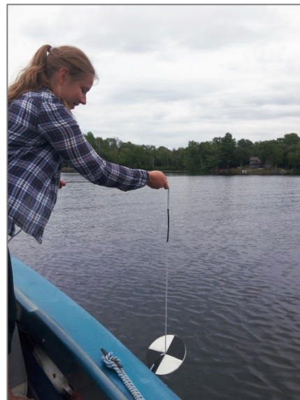
Figure 4: Using a Secchi disk.
