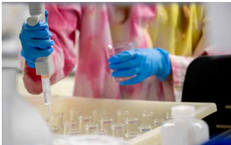
Figure 2. Georgia Bunnell prepares a set of total phosphorus samples to be analyzed.
