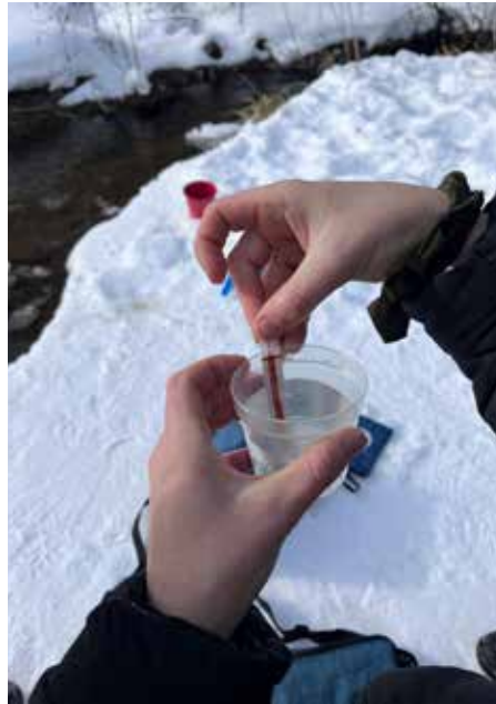
Figure 1. Lake Erie Rangers winter road salt chloride test strip.
